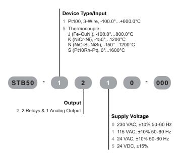
The STB55 safety temperature limiter is used as a behind panel device when thermal processes must be monitored and the system must be transferred into a safe operational state in case of fault.
