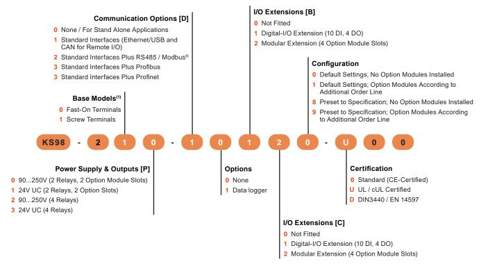
(1) Universal Input, 2 digital inputs, TPS, 2 option module slots
