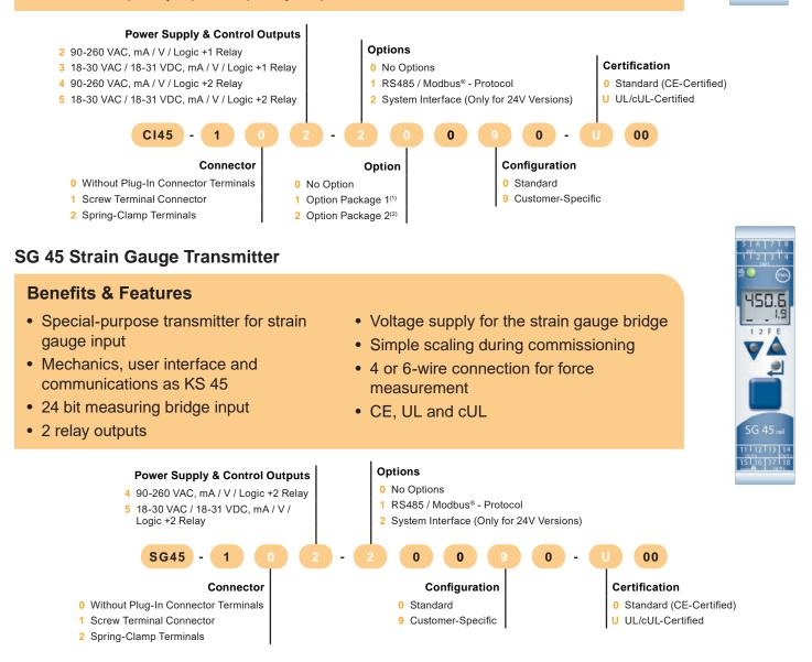
(1) Option package 1: additional universal input INP2, plus: O2-measuring; counter input; functions tare, sample & hold and integrator <sup>(2)</sup> Option package 2: additional to option package 1: digital input as optocoupler and frequency input / output
